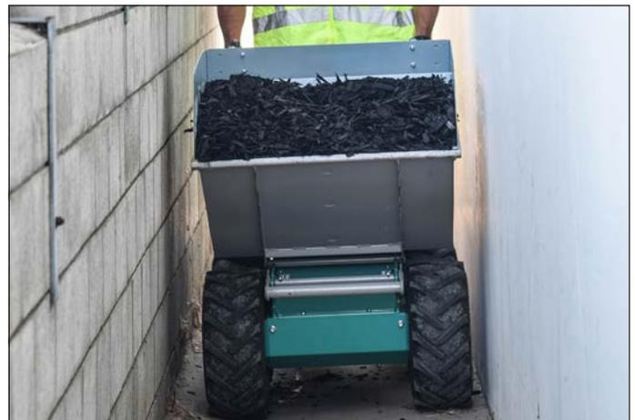
**Optional 2.8 ft<sup>3</sup> steel clip-on tub — TT7 —** allows access through narrow 32-inch passageways.
