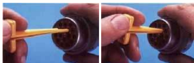
Figure 7-9 HD/HDP contact removal
