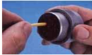
Figure 7-7 HD/HDP contact installation
