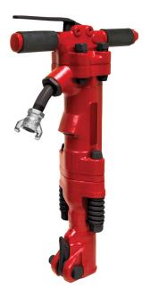
60 LB Class Thor Style Pavement Breaker. Hard hitting 60 lb. class tools for heavy demolition work. Designed for ripping out reinforced concrete and tearing out streets. Features rubber hand grips for improved operator comfort and a swivel hose connection. Durable, rugged pistons for extremely versatile demolition purposes.
