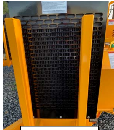
RADIATOR SCREEN - CLEAN FROM THIS SIDE
