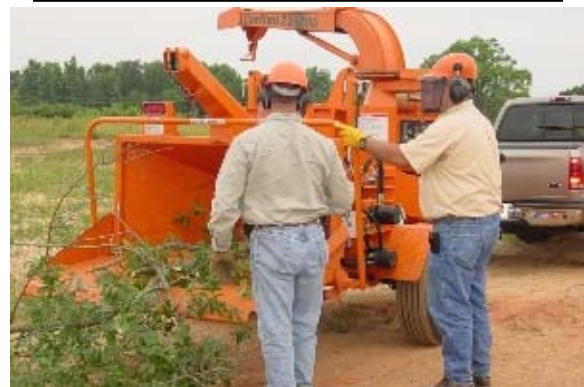
ALWAYS FEED MATERIAL FROM THE RIGHT SIDE AND BUTT END FIRST
