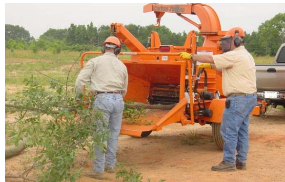
ALWAYS FEED MATERIAL FROM THE RIGHT SIDE AND BUTT END FIRST
