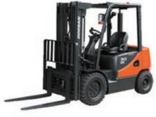
4-wheel, LPG/Diesel pneumatic tire
