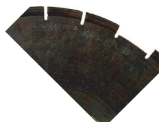
Segment Loss: Usually insufficient water
