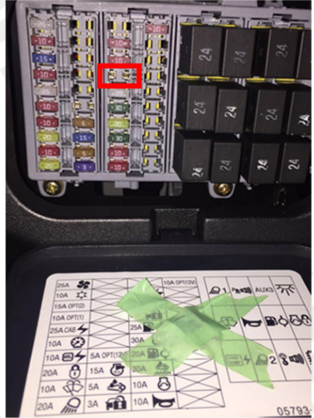
TB2150 Uninstall Fuse Example Cover Open
