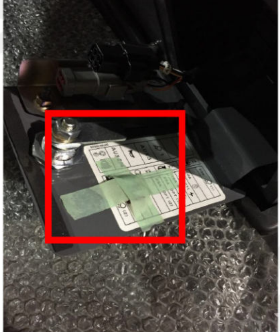
TB230 TB240 TB260 Uninstalled Fuse Example Cover Open
