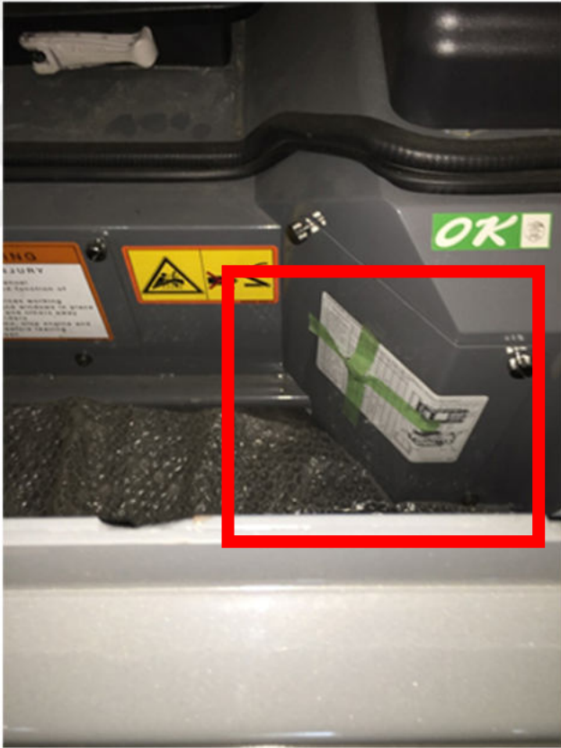
TL10V2 TL12R2 TL12V2 Uninstalled Fuse Example
