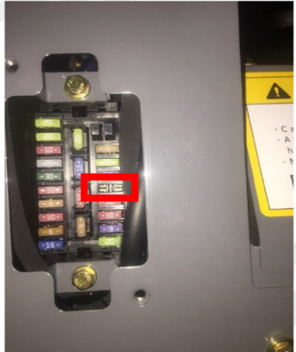
TL10 TL12 Uninstalled Fuse Example Cover Open
