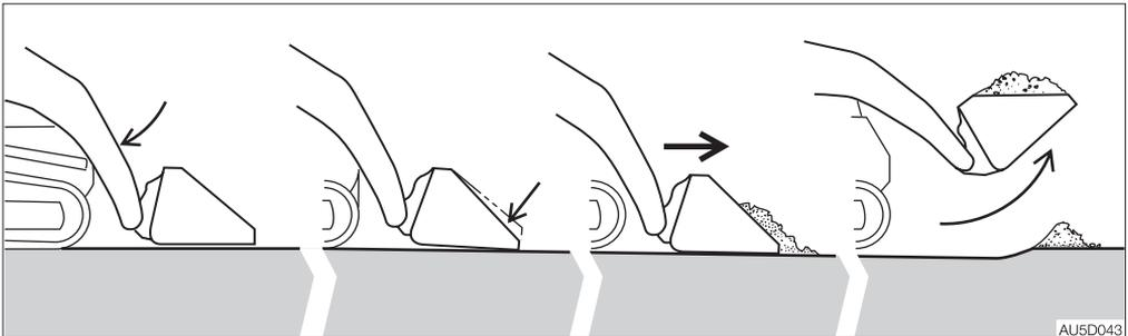
Tilt the bucket forward at an angle appropriate for the ground hardness. Slowly travel forward, dig into the ground with the cutting edge of the bucket. When the bucket is full, tilt it backward.
