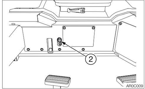
2. Press the lift arm lower button (2) to lower the lift arm.
