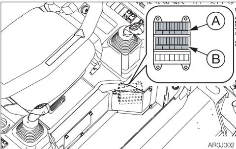
2. Loosen the screw and remove the fuse box cover (1).
