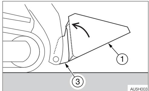
5. Tilt the quick-hitch (3) backward while lifting the bucket (1) off the ground. The quick-hitch (3) will slide into position.
