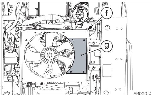
5. Remove the plate (g) from the fan shroud (f).
