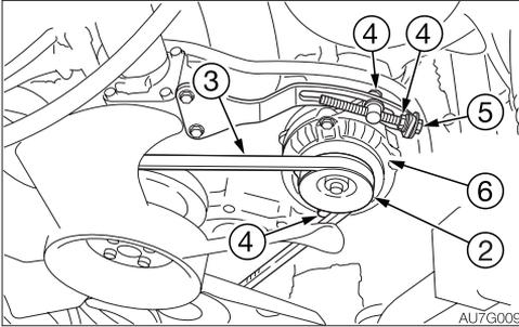
1. Loosen the lock nuts (4).
