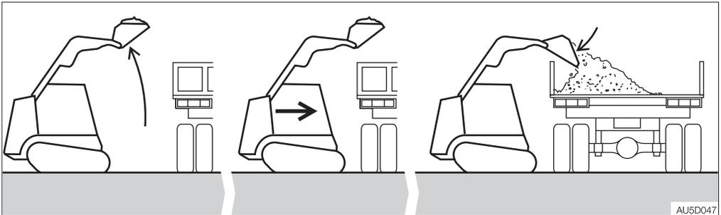
Move the machine, stop close to the truck, and then raise the bucket until its lower edge is well above the truck bed. Slowly move the machine forward and stop at the position where the bucket is to dump. Tilt the bucket forward to release the material in the bucket into the truck bed. When the truck bed is filled to half capacity, use the bucket to spread the load evenly.
