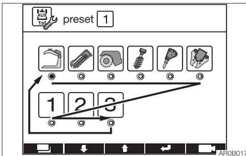
Pressing the Enter key while the cursor ► is at "ATT" goes to the attachment select screen. Pressing the Down (↓) key moves the cursor ● in the direction of the arrow. Use the Up (↑) key to move the cursor ● in the opposite direction of the arrow. Move the cursor ● to the desired symbol or the number, and then press the Enter key to confirm. The selected symbol will appear at the lower left of the Home screen.
