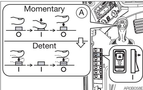
**IMPORTANT:** Do not operate the machine in the detent mode for a long time. Doing so will increase the hydraulic oil temperature and shorten the service life of the hydraulic units.
