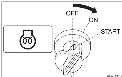
1. Turn the ignition key to the ON position, and confirm that the glow lamp is lit. (The glow lamp stays lit while the coolant temperature is kept at 0°C (32°F) or lower.)
