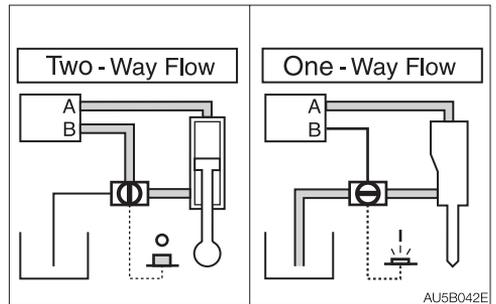
To set the auxiliary line flow to the one-way mode, press the ON side of the switch until the auxiliary 1st one-way indicator lamp lights up. To change it to the two-way mode, press the OFF side of the switch until the auxiliary 1st one-way indicator lamp goes out.
