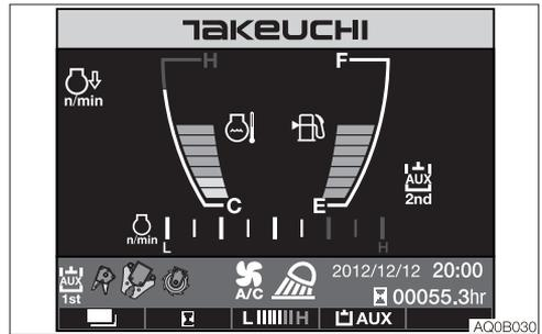
Turn on the light switch on any screen to decrease the display brightness and to enter the “evening mode”.
