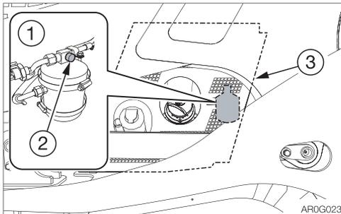
1. Loosen the bolts and remove the cover (3).
