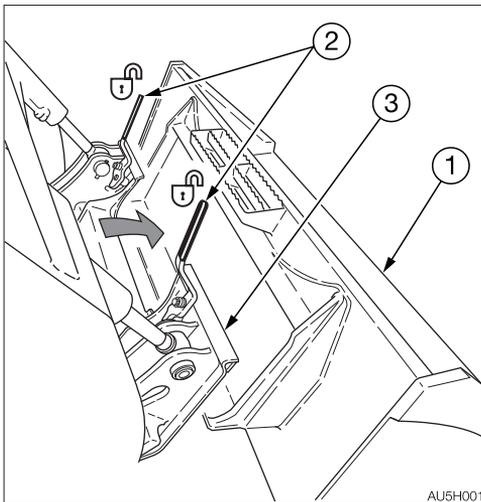
1. Make sure the quick-hitch (3) lock levers (2) are in the unlock position.
