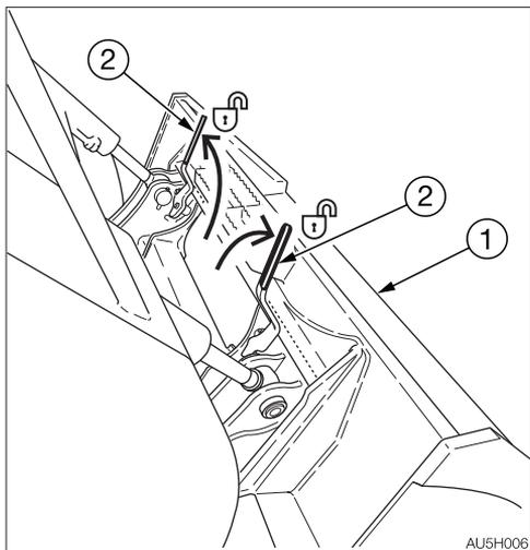
3. Pull both lock levers (2) until they are vertical to release the latch.
