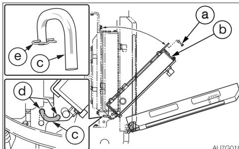
2. Remove the bolts (a) and open the radiator (b).
