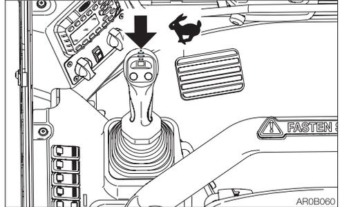
Press this button to set the travel speed to 2nd (high) speed. Press it again to return to 1st (low) speed.
