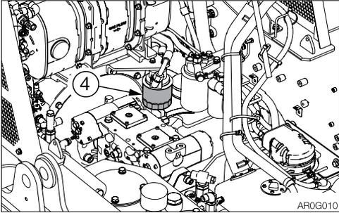
10. Turn the filter (4) counterclockwise with the filter wrench and remove it.
