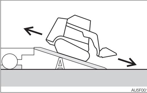
6. When getting on or down the ramps, the bucket must be pointing down the slope.
