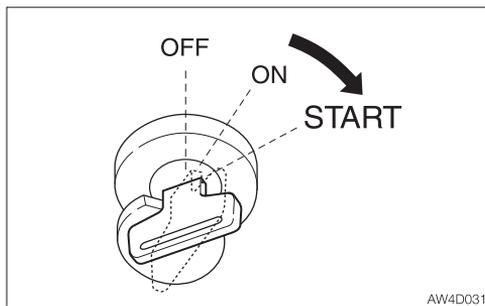
1. Turn the ignition key to the START position and start the engine.
