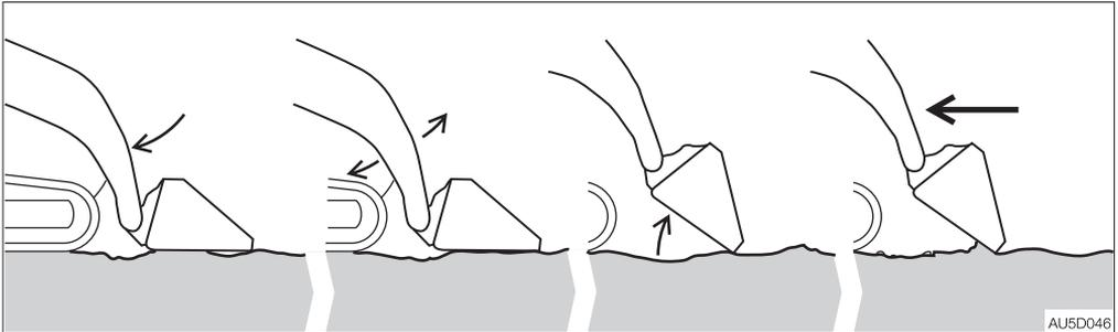
Lower the bucket to the ground before setting the lift arms to the float mode. Tilt the bucket forward to stand it on its cutting edge, and then level the loose ground while driving in reverse.
