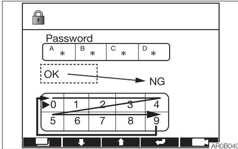
When the “closed-lock” symbol is displayed, it is necessary to enter the password to set the auxiliary flow rate, lock/unlock the auxiliary flow rate or change the password. Move the cursor ► with the Up (↑) or Down (↓) key, and press the Enter key to enter a 4-digit number password. Enter the existing password. If it is correct, “OK” will be displayed followed by the setting screen. If it is not, “NG” will be displayed followed by the machine setting screen.
