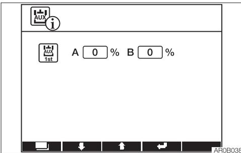
Displays the flow rate of the Auxiliary 1st, 2nd and 4th.
