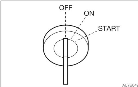
**IMPORTANT:** Do not repeatedly switch the key from OFF to ON and ON to OFF over a short period. Doing so will cause engine breakdown.
