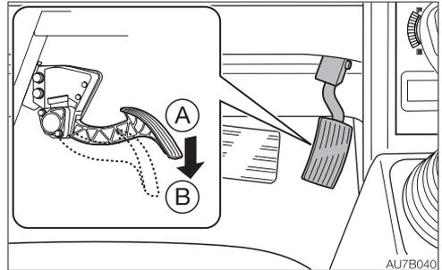
This controls the engine speed.
