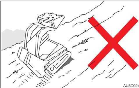
Do not travel or turn with the bucket raised. Keep the bucket as low as possible during traveling.
