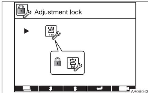
It is possible to request the user to enter a password when setting the auxiliary flow rate.
