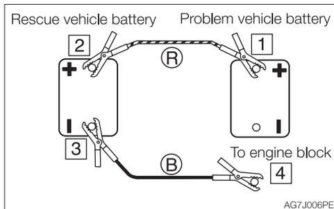
1. Connect the clip of jumper cable (R) to the positive (+) battery terminal of the dead machine.
