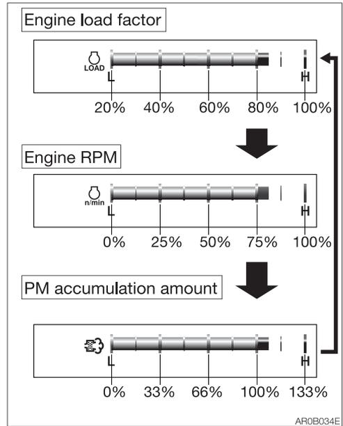
This gauge displays the load condition of the work. When the gauge is in the green range, the work load is light to medium. When the gauge is in the red range (75% or more), the work load is high. When the button (C) (Bar meter key) is pressed on a normal screen, the display changes in the following order: the engine load factor, throttle opening position and PM accumulation amount indicator.
