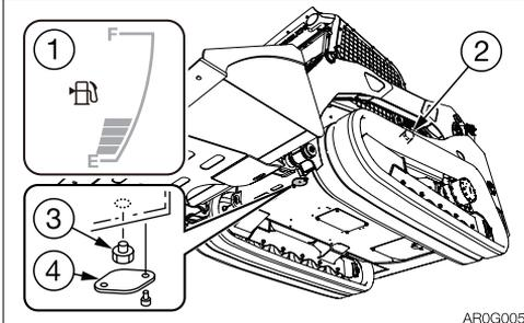
1. Check the fuel level using the fuel gauge (1).
