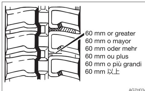
Repair if there are cracks of 60 mm (2.4 in.) or greater in length.
