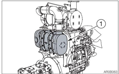
6. The regeneration promoting indicator lamp changes from flashing to solid, indicating that the engine RPM is automatically increased and the DPF (1) regeneration (PM burning) is started.
