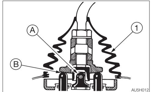
1. Remove the lower mount section of the boot (1) and turn it upward.
