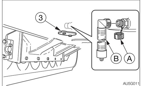
5. Loosen the bolts and remove the under cover (3).
