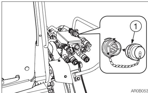
1. Turn the cap (1) counterclockwise and remove it.
