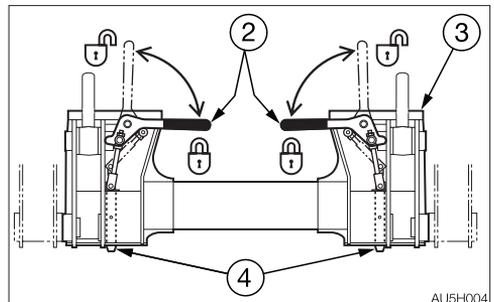
8. Push both lock levers (2) until they are horizontal to engage the latch.
