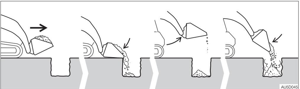
With the bucket lowered, drive near the hole and tilt the front edge of the bucket downward as soon as it passes over the near side of the hole. Raise the bucket and empty the load only when necessary.
