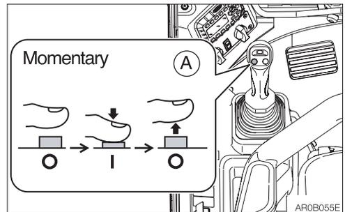
These switches stay on while the buttons are pressed; they turn off when the buttons are released (momentary mode).
