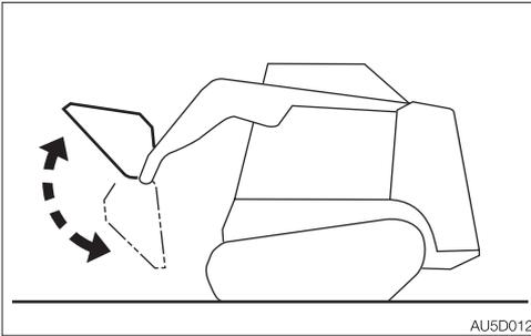
2. Set the bucket cylinder at the stroke end and keep it there. Do not keep this condition for more than 30 seconds.
