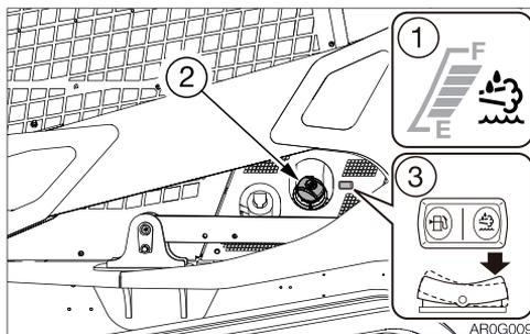
Use the DEF/AdBlue® level indicator to check the amount of DEF/AdBlue® solution remaining.
