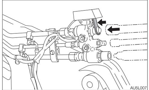
**Note:** This device works as a safety device to prevent accidental activation of the attachment or hydraulic quick-hitch installed. When the attachment hoses are connected to the quick-coupler, the plate is pushed to turn on the switch, which prevents the hydraulic quick-hitch from being activated even when the lock/unlock switch on the hydraulic quick-hitch is pressed. When the hydraulic quick-hitch needs to be activated, disconnect all hoses from the quick-coupler.
