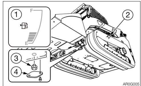
1. Remove the fuel filler cap (2).
