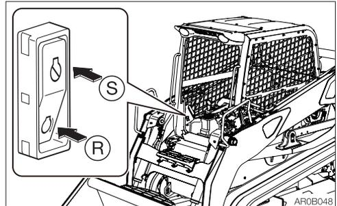
This switch is used to shutdown the engine if it fails to stop, due to machine failure or breakage, when the ignition switch is set to the OFF position.
