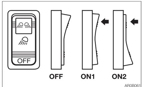
When this switch is turned while the ignition switch is at ON, the lights turn on as follows:
