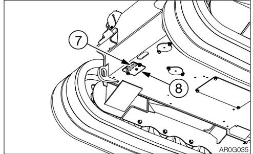
2. Place a pan for catching the waste oil under the drain plug (7).
