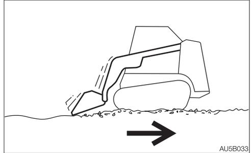
While in the float mode, the bucket moves up and down in response to the “bumps and dips” on the ground surface.
