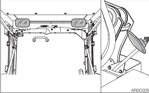
Adjust the rear view mirrors to have a better rear view.
