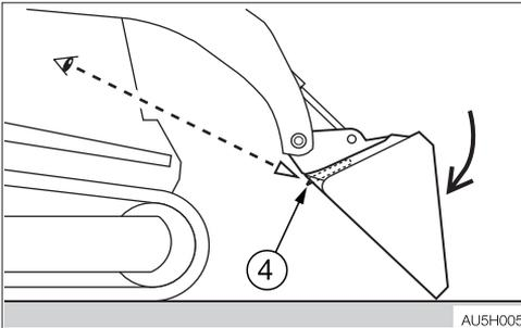
7. Check that the tips of the pins (4) are projecting through the bracket hole on the bucket to indicate that the latch is properly engaged.
