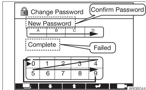
The password can be changed. Use the Up (↑) or Down (↓) key to move the cursor ► to the password field, and then press the Enter key to enter a 4-digit number password.
