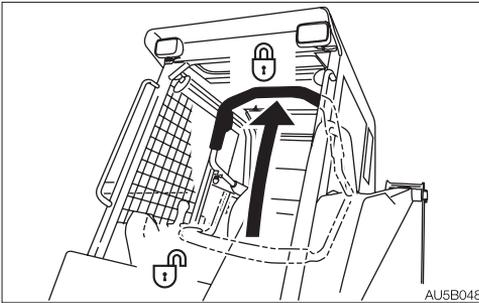
This device is used to lock the functions of control levers and switches listed below.
