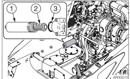
2. Turn the case (1) counterclockwise and remove it.
