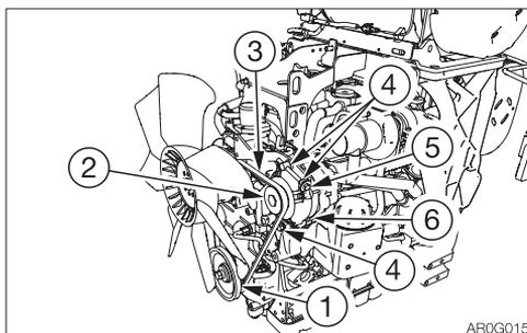
6. Press on the belt at the midpoint between the crank pulley (1) and alternator pulley (2) to check the tension (approx. 98 N or 22 lbf).
