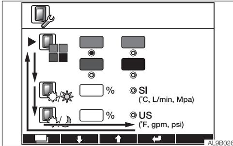
The display settings can be changed. Use the UP (↑) or Down (↓) key to move the cursor ▶.
