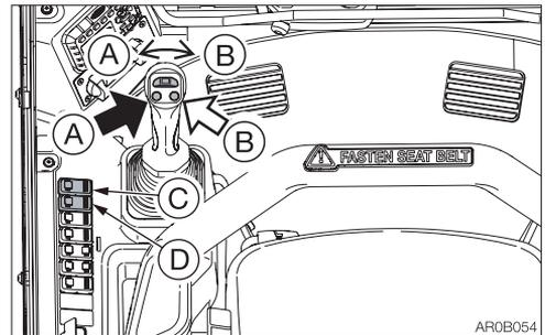
Press auxiliary hydraulic buttons (A) or (B) to control the flow of the oil in the auxiliary hydraulic circuit.
