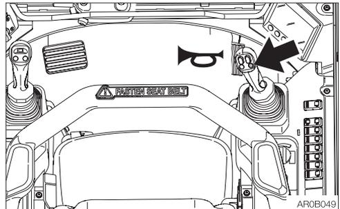
Press the button situated on the right operating lever to blow the horn.
