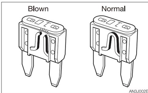
4. If a fuse is blown, replace it with a spare fuse of the same capacity.
