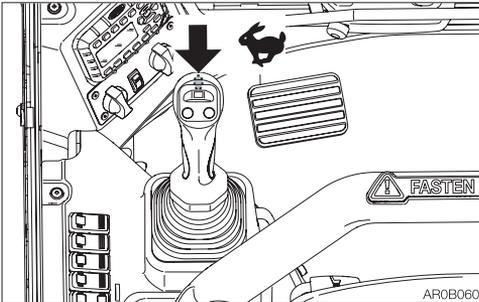
Press the travel speed button on the left control lever to switch to 2nd (high) speed, and press it again to return to 1st (low) speed.
