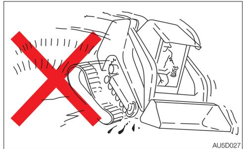
Do not attempt a spin turn or pivot turn at high speeds. Doing so may cause the machine to tip over or the tracks to come off and/or extremely wear.
