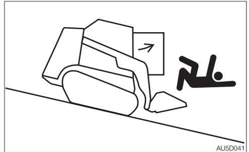
Opening the door while traveling on slopes is dangerous, as the force required to open and close the door changes abruptly. Always keep the door closed when traveling on slopes.
