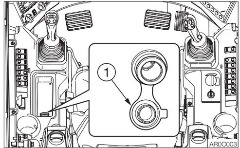
Use this socket to connect the external power supply. When using, be careful not to exceed 12V/5A.
