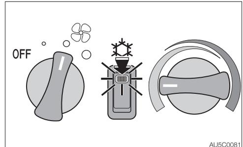
1. Set the desired temperature by turning the temperature control dial to between the center and COOL.
