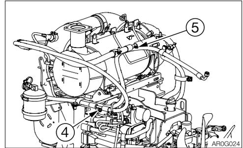
5. Check the temperature of the compressor's high pressure pipe (4) and low pressure pipe (5). Refer to "Check list for refrigerant volume" on page 5-45.
