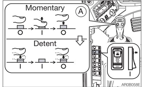
2. Select the operation mode for the auxiliary hydraulic button (A) by operating the detent mode switch (D).
