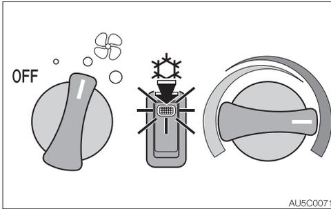
1. Set the desired temperature by turning the temperature control dial to between the center and HOT.
