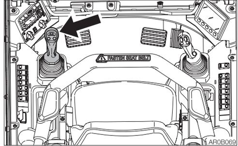
Use this lever to move forward and in reverse and to change directions.
