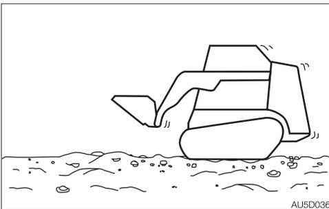
On uneven ground, maintain the low speed and avoid starting, stopping or changing directions abruptly.
