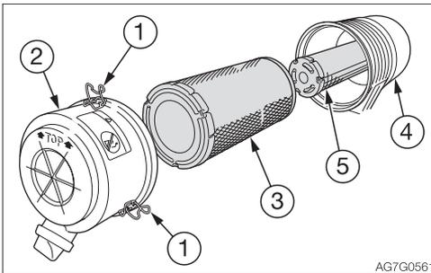
2. Loosen the clamps (1) and remove the dust cup (2).
