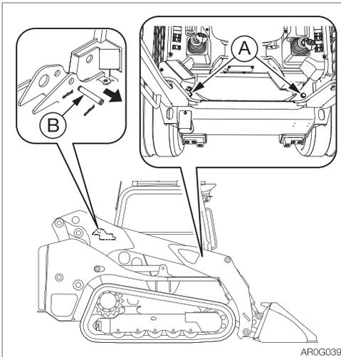
1. Select a firm, level surface, set the machine to the posture shown in the diagram above, ground the working equipment, then stop the engine.
