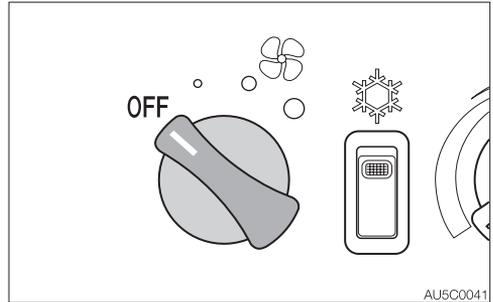
Use this switch to adjust the fan speed in three steps. Turning to the OFF position turns off the air conditioner.
