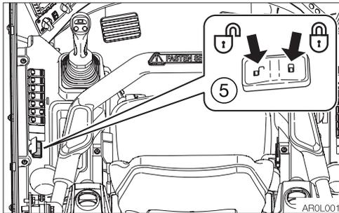
2. Open the cover and press the
