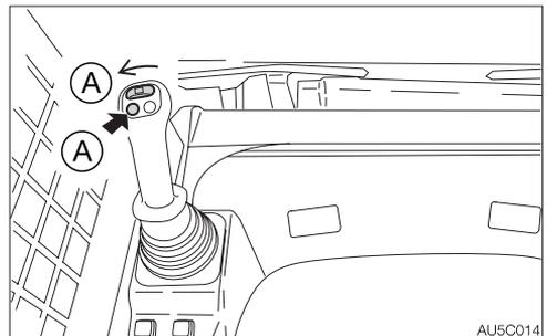
2. Press the auxiliary hydraulic button (A) or slide the slider switch to the left side (A).
