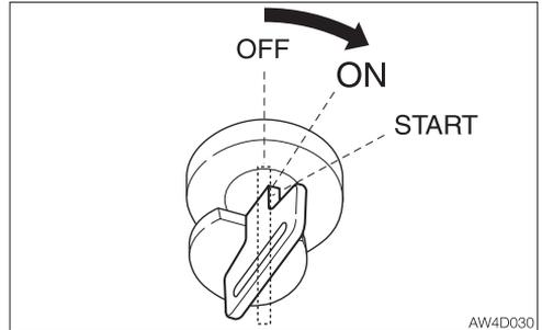
4. Turn the ignition key to the ON position and hold it for about 60 seconds.
