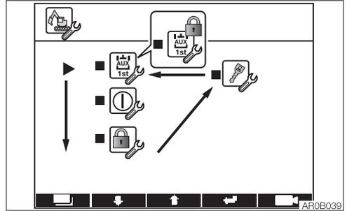
The settings made to the machine can be changed. Move the cursor ► with the Up (↑) or Down (↓) key to go to the desired item to be set, and then press the Enter key to confirm.
