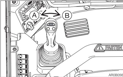
Proportional control allows for slow-to-fast movement of auxiliary functions.
