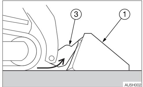
4. Slowly move the machine forward and raise the lift arms. Engage the wedge-shaped top edge of the quick-hitch (3) onto the bucket (1) upper part (quick-hitch mount).
