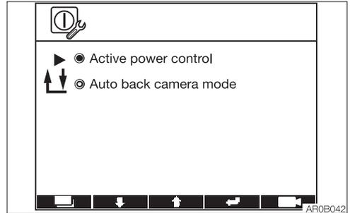
The active power control and the auto rear view camera mode can be set to ON or OFF. To return to the machine setting screen, press the Menu key. Use the Up (↑) or Down (↓) key to move the cursor ►, and then press the Enter key to turn on or off the blue circle. Blue circle is lit: ON
