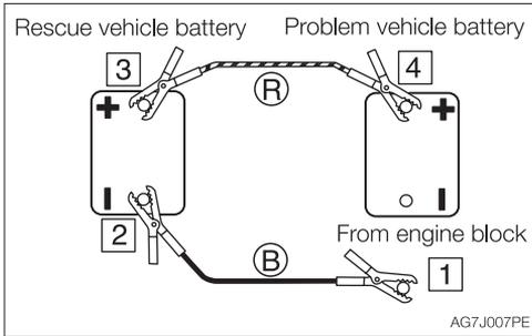
1. Disconnect the clip of jumper cable (B) from the engine block of the dead machine.
