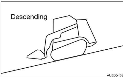
If the engine stops when descending a slope, set the left control lever to the neutral position, stop the machine, then start the engine.
