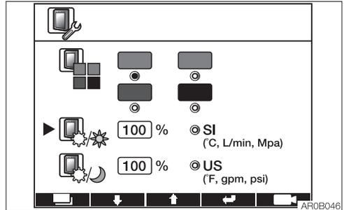
The brightness of the LCD is set to between 20 and 100%.
