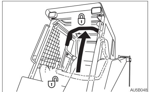
3. Raise the safety bar to the locked position, and then check that the control levers are locked.
