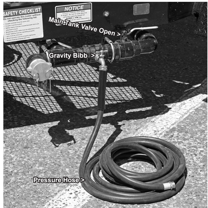
Figure B15 Gravity Flow Hose Connection
