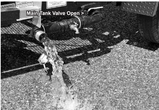
Figure C1 Main Tank Drain
