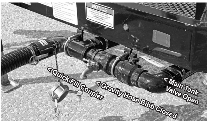
Figure B4 Filling Tank From Pressurized Source
