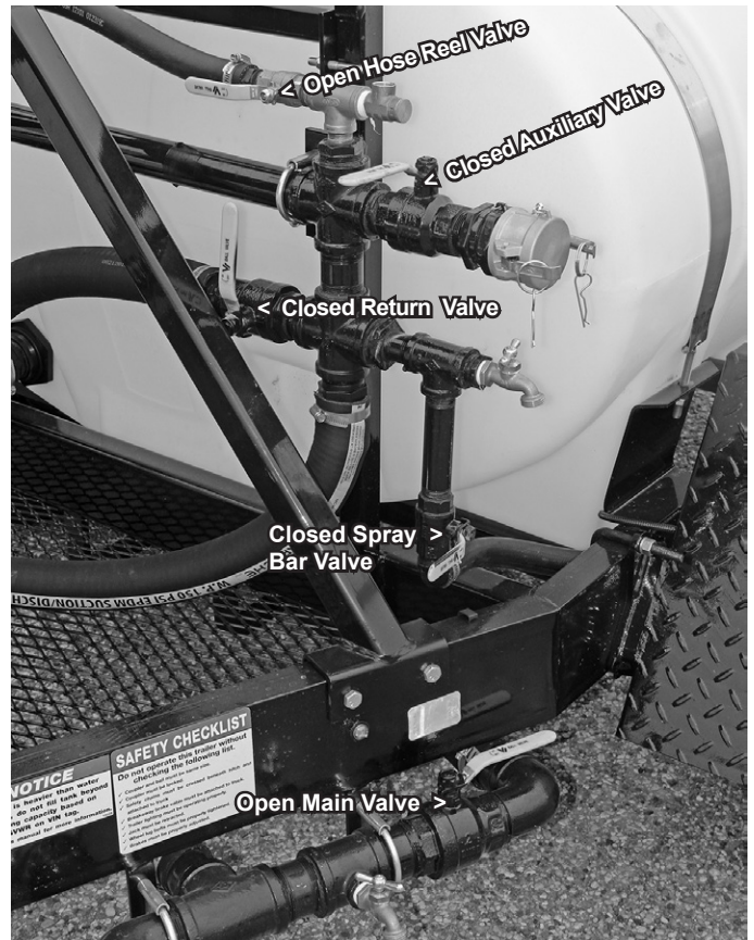
Figure B25 Valve Setting for Hose Reel Operation
