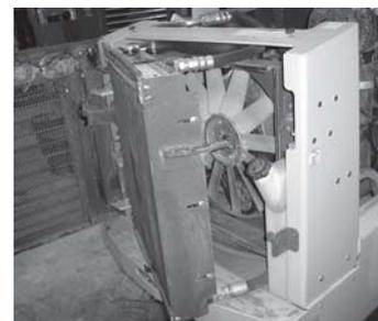
**Fig. 51: Swing cooler out**
