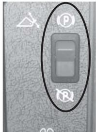
Fig. 3: Parking Brake Switch
