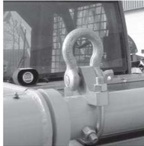
Fig. 35: Four-Point Lift Rear Lift Eye
