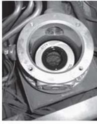
**Fig. 49: Hydraulic Oil Filter**
