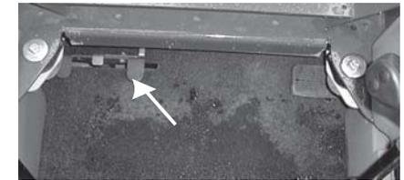
Fig. 21: T-Bar, Dual-Hand and Joystick Auxiliary Hydraulic Control
