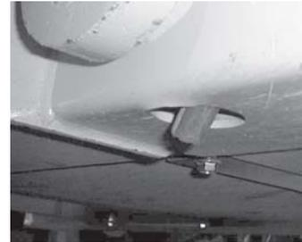
**Fig. 47: Remote Engine Oil Drain**
