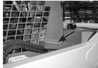
Fig. 5: Lift Arm Support Device Storage Location
