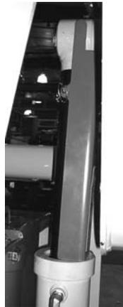
Fig. 4: Lift Arm Support Device Engaged
