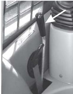
**Fig. 8: Hand Throttle Lever (Joystick controlled units)**
