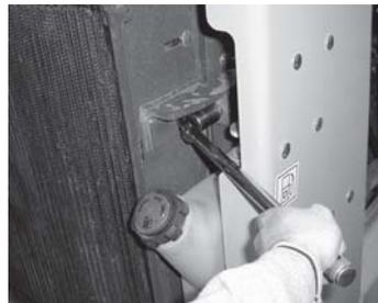
**Fig. 50: Remove cooler lock bolt**
