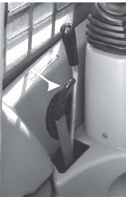
**Fig. 24: High-Flow Control (Joystick controlled units)**
