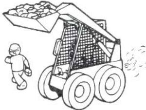
**!** Never leave loader with engine running or with lift arm up. To park, engage parking brake and put attachment flat on the ground.
