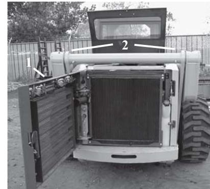
**Fig. 38: Engine Compartment Access Doors**
