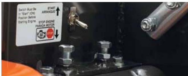
Start/stop switch on gasoline powered Guardmatic®.
