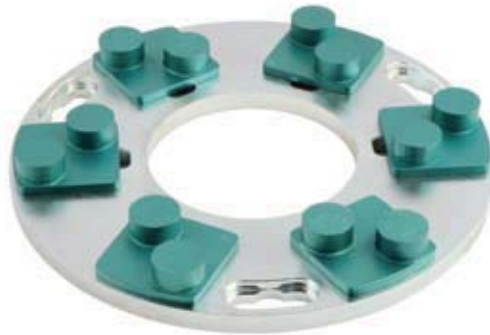
Low-profile disc holder and recessed locking mechanism reduces overall height of tooling to keep the machine closer to the ground. This reduces the cavity size under the grinder and increases efficiency of dust extraction.
