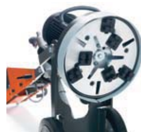
Single grinding plate with multiple diamond tool distribution positions.
