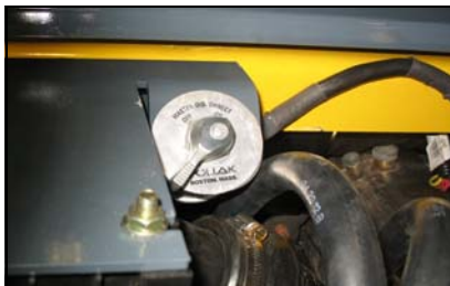
Figure 14 – Battery Disconnect Switch
