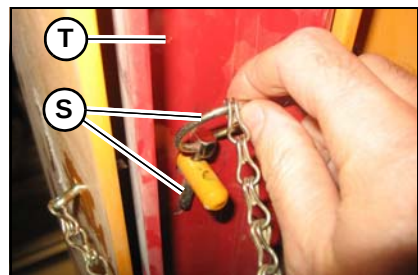
Figure 11 – Lift Arm Support Storage Lynchpin Removal
