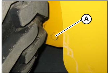
Figure 95 – Model R165 Remote Engine Oil Drain Plug Location
