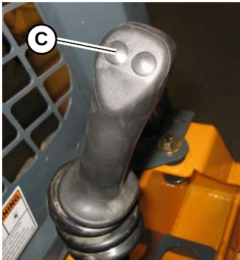
Figure 34 – Two-Speed Drive Control Button
