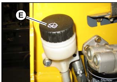
Figure 117 – Windshield Washer Reservoir Fill
