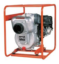
4" Suction / 4" Discharge 425 GPM Flow 100' Head (43.3 psi) HONDA GX240, 7.9HP
