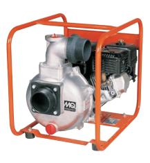
3" Suction / 3" Discharge 245 GPM Flow 98' Head (42.4 psi) HONDA GX160, 4.8HP **QP402H**
