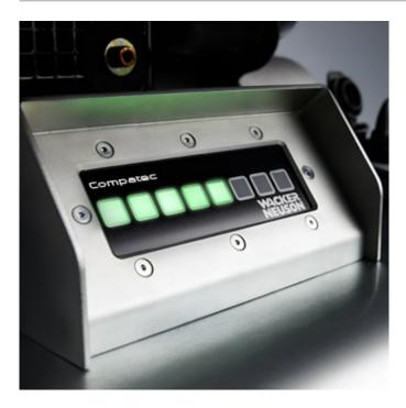
Compatec - Compaction Control **Available as an accessory**: Easy to read Compatec helps the operator determine when maximum compaction has been reached. The number of lights will increase with each pass and no longer increase once maximum compaction is achieved Retro-Fitting for DPU 4545 He are also available.
