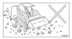
Traveling or slewing on broken stone, jagged base rock, iron rods, iron scraps or the edges of iron sheets may damage or cut the crawlers.
