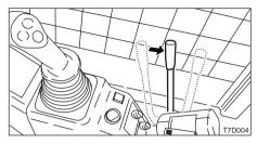
Pull the throttle lever to the middle speed position.
