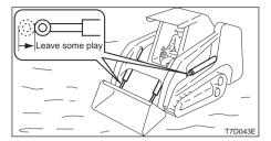
Do not conduct operations with the cylinders fully extended or retracted. Doing so applies excessive force on the cylinders and may damage them.
