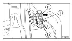
1. Connect the attachment hydraulic lines to ports (a) and (b).
