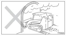
Do not use this loader in areas where there is danger of explosion from volatile gases. Also avoid using the loader where the exhaust gases could come in contact with flammable items.
