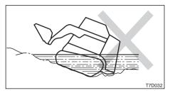
If you leave water at a sharp angle, the rear of the machine may be submerged, exposing the radiator fan to water and damaging them. Do not let the rear of the machine get submerged.
