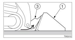
Move the machine slowly forward and raise the loader lift arms. The wedge shaped top edge of the quick attachment (3) must engage in the upper mounts of the bucket or attachment.
