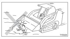
Hitting the bucket against rocks, etc., could damage the bucket or the bucket cylinder.
