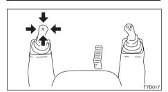
Slowly set the left control lever to the neutral position. The machine stops.
