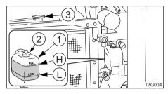
2. Gradually loosen the radiator cap (3) to release the internal pressure, then remove.
