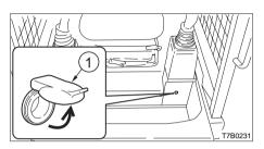
Use this socket as an external power supply. When using this socket, be careful not to exceed 12V/5A.
