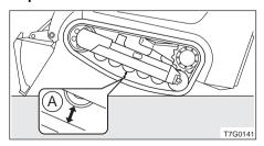
Lower the lift arm and tilt the bucket forward to raise the front of the loader off the ground as far as it will go. Measure the clearance between the center track roller and the surface of the crawler belt where it makes contact with the roller.
