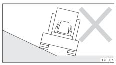
Avoid traveling with one crawler on a slope or projecting object and the other crawler on a flat surface (with the machine at a tilt of 10° or greater). Travel with both crawlers on flat surfaces.
