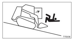
Opening the front door while traveling on slopes can be hazardous, because the force required to open and close the door changes abruptly. Always keep the door closed when traveling on slopes.
