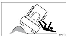
Traveling over obstacles (rocks, stumps, etc.) may subject the body to strong shocks and result in damage. Avoid traveling over obstacles whenever possible. If you must do so, keep the bucket near the ground, travel at low speed, and go over the obstacle at the center of the crawler.
