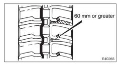
Repair if there are cracks of 60 mm (2.4 in.) or greater in length.
