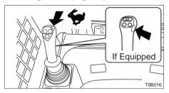
Press the travel speed switch on the left control lever to switch to 2nd (high) speed, and press it again to return to 1st speed (low speed).
