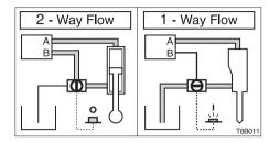
Change the direction of the hydraulic oil flow by setting Flow selector switch (C) ON to return the oil in the (b) port line directly to the hydraulic tank.
