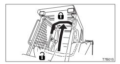
3. Set the safety bar to the locked position and check that the control levers, auxiliary pedal are locked.
