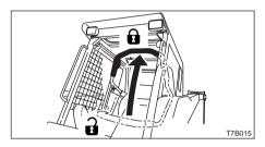
3. Check that the safety bar is in the locked position.
