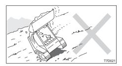
Work should not be performed on a slope since the balance of the machine can be lost when operating the working equipment and there is the danger of the machine tipping over.
