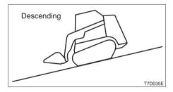
If the engine stops when traveling down a slope, set the control levers and pedal to the neutral position, stop the machine and restart the engine.
