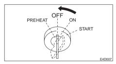
2. Turn the key to the OFF position to stop the engine.
