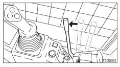
Return the throttle lever, then idle the engine and run it for about 5 minutes with no load.
