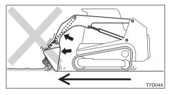
Do not perform scooping or grading operations with the bucket cylinders fully extended. The traction force will apply extremely heavy loads on the bucket cylinders and this may damage them.
