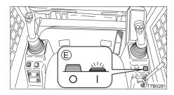
2. Turn on the High Flow switch (E) (green light is ON).
