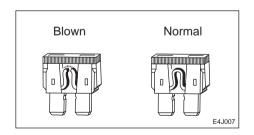
4. If a fuse is blown, replace it with a spare fuse of the same capacity.
