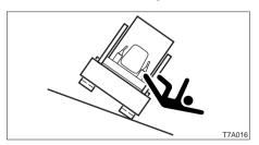
Do not change directions or cross slopes sideways. First return to a flat surface then redirect the machine.  On grass, dead leaves, wet metal or frozen surfaces, the machine may slide sideways even on very gentle slopes.
