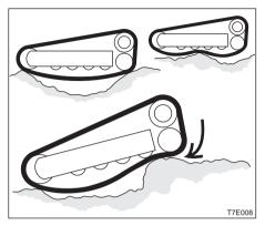
• Do not change directions when the crawler belts are slack as shown in the diagram.
