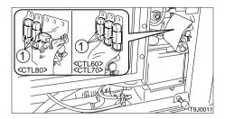
If the power is not switched on after turning the starter switch to the ON position, the cartridge type fusible links (1) might be blown open. Open the rear door and inspect. If the fusible link is blown, please contact your dealer.
