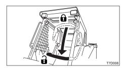
2. Set the safety bar to the released position and lift the bucket from the ground.
