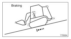
Braking is automatically applied by the hydrostatic drive system when the left control lever is returned to the neutral position. Full braking is achieved when the safety bar is raised.
