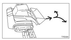
When traveling up large cobblestone or rock steps (20 cm (8 in.) or greater), climb up the step at a direct angle and do not change course on top of the step.
