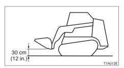
Rollback the bucket fully and lift the bucket to 30 cm (12 in.) above the ground.
