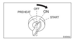
2. Turn the starter key to the ON position and hold it there for about 20 seconds.
