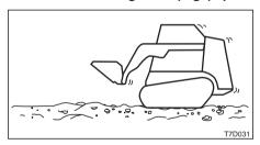
On uneven ground, travel at low speed and avoid accelerating, stopping or changing directions abruptly.
