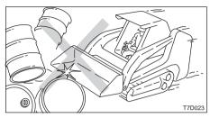
Travel at a speed which is appropriate for the conditions. Travel at low speed when the field of view is obstructed and take extra precautions with hazardous materials.
