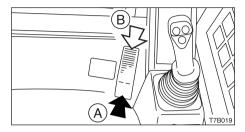
Use this pedal to operate the auxiliary hydraulics circuit.
