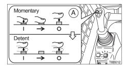
One press of the auxiliary hydraulic switch (A) sets it to ON and one more press sets it to OFF. There is no need to continue pressing the switch.
