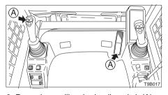
Press the auxiliary hydraulic switch (A) or press the heel side (A) of the pedal.
