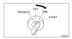
Insert the key into the starter switch, turn it to the ON position, then perform the following inspection:
