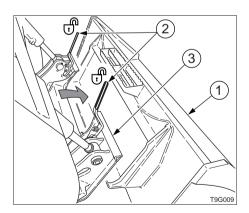
2. While sitting in the operator's seat with the safety bar down, start the engine and tilt the quick attachment (3) forward.
