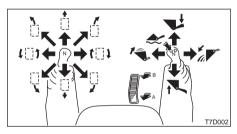
4. Check that the control levers and pedals are in the neutral position.
