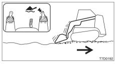
→ To floating the lift arms: Press the float switch on the right control lever.
