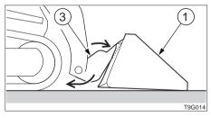
5. Rotate the quick attachment (3) out (bucket dump function) allowing the bucket or attachment to slide off the top edge of the quick attachment (3).
