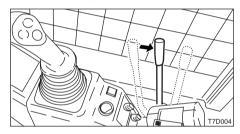
1. Pull the throttle lever to the middle position.
