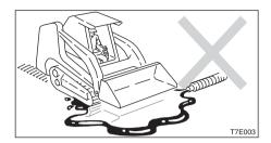
Do not let fuel, oil, salt or chemical solvents get on the crawlers. These substances may corrode the couplings of the crawlers' metal cores, resulting in rust or peeling. If these substances should get on the crawlers, wipe them off immediately using water.
