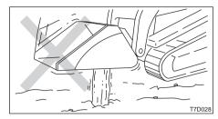
Do not use the downward force of the bucket to drive piles.
