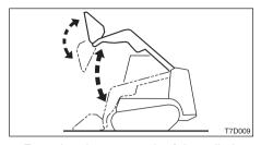
3. Extend and retract each of the cylinders several times with no load.
