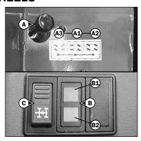
This switch enables alignment of the wheels. The indicator lamp indicates if it is ON.
