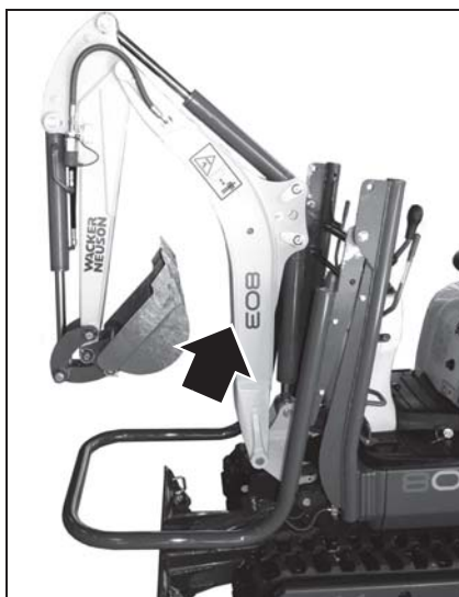
Fig. 88: Lowering the rollbar
