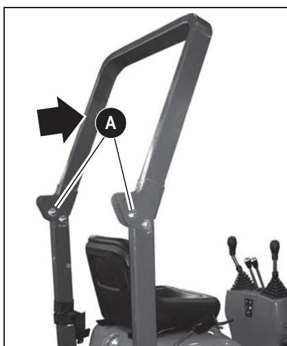
Fig. 84: Raising the rollbar
