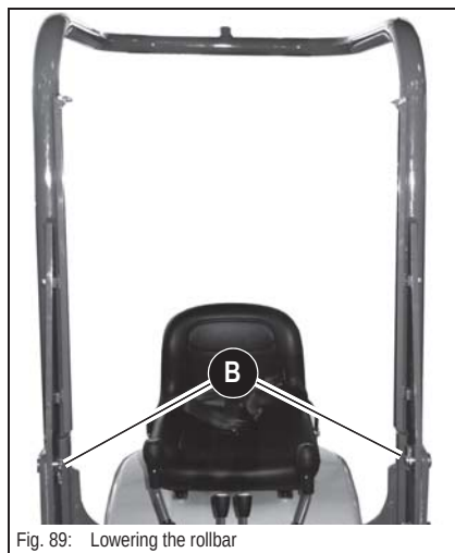
Fig. 89: Lowering the rollbar
