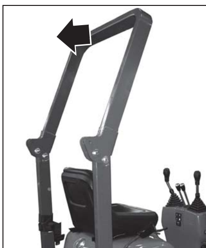
Fig. 83: Lowering the rollbar
