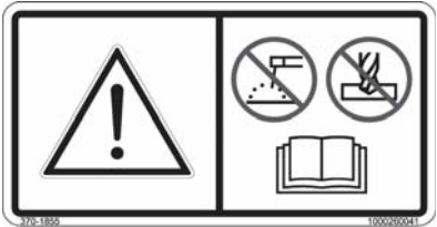
Fig. 39: Do not drill holes or weld the ROPS structure
