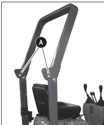
Fig. 82: Lowering the rollbar
