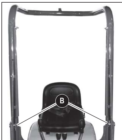
Fig. 86: Lowering the rollbar
