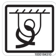
Fig. 10: Slings points for tying down the machine
