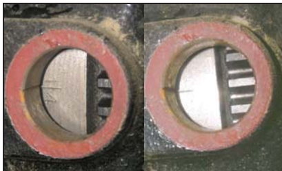
Fig. 7: Top dead centre indentation and 10° before top dead centre
