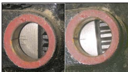
Fig. 8: Top dead centre indentation and 10° before top dead centre
