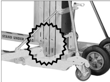
Pull the tool down and the brake will release.
