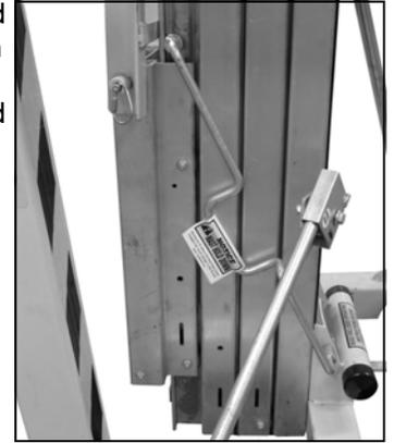
The winch handles have been placed in the stored position.
