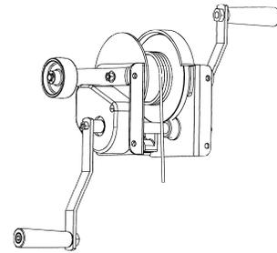
10. Wind the slack cable tightly and evenly across the load drum.
