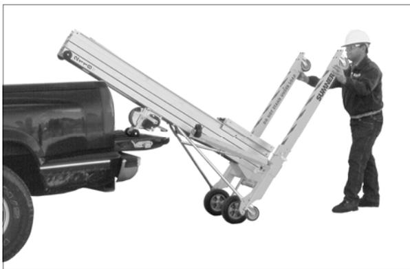
**IMPORTANT** Before tilting unit to reclined position, the carriage must be lowered all the way down and the Carriage Safety Latch must be engaged.
