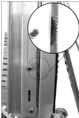
When the brake is engaged, it will be possible to see the Brake Cam acting on the adjacent mast section. Once the brake is released, it will rotate around into its normal position and will not be visible.
