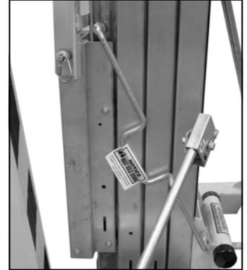
To release Hold Down, pull bar toward you and place back behind mast sections.
