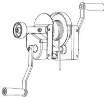
If cable is kinked, worn, frayed, damaged, or has anything on it that would obstruct its rotation around the pulley wheels, **do not use the unit!**
