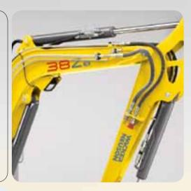
The innovative hydraulic EASY LOCK quick-hitch system is optimally suited to the kinematics of Wacker Neuson compact excavators and makes a decisive contribution to work process improvement. Just drive up, hook up and lock automatically. Its low headway means that the bucket displacement angle remains unaffected. Workflow improvement is guaranteed.
