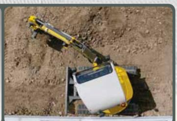
The unique construction principle of the Wacker Neuson Zero Tail machines.
